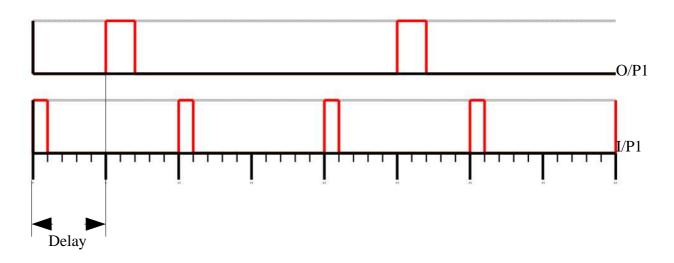
In the above example the divide value has been set to 2 so that one output is generated for every two inputs. Note that there is also a Delay value set so that the output pulse is shifted in relation to the input pulse.
