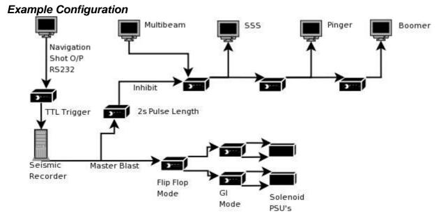
The above diagram shows how a number of Universal trigger box's may be connected together to form a complete integrated survey system for single pass operations, using High Resolution Seismic, Multibeam Sonar, Side Scan Sonar, Pinger and Boomer systems. Other systems that may be integrated include single beam echo sounders, Doppler velocity logs, and acoustic navigation / tracking systems.
